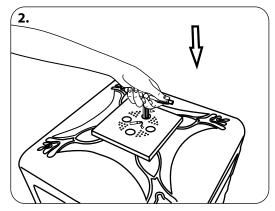
Push the plunger down through the aperture.
