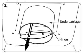
The plunger will push the trapdoor open to empty the contents of the ashtrays undercarriage into the main liner of the litter bin.
