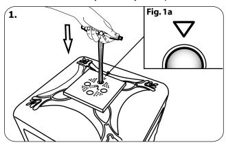
To empty the ashtray the plunger must be inserted into the hole marked with an arrow (see Fig. 1a).
